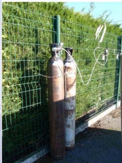
Tanks connected to nitrogen flux (minimization of volatilization)
