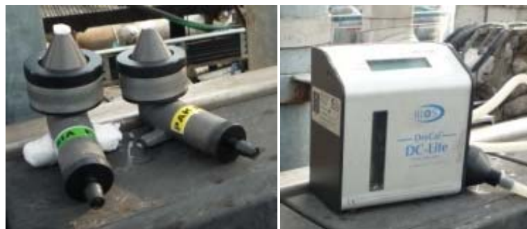
Figure 2 Photographs of BIA cassette and sampling pump calibration device A - BIA Sampling cassette B - Sampling pump calibration device
