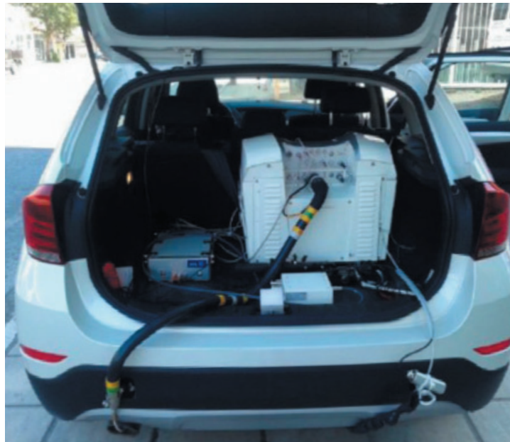
Figure 5 PEMS installation on the vehicle
