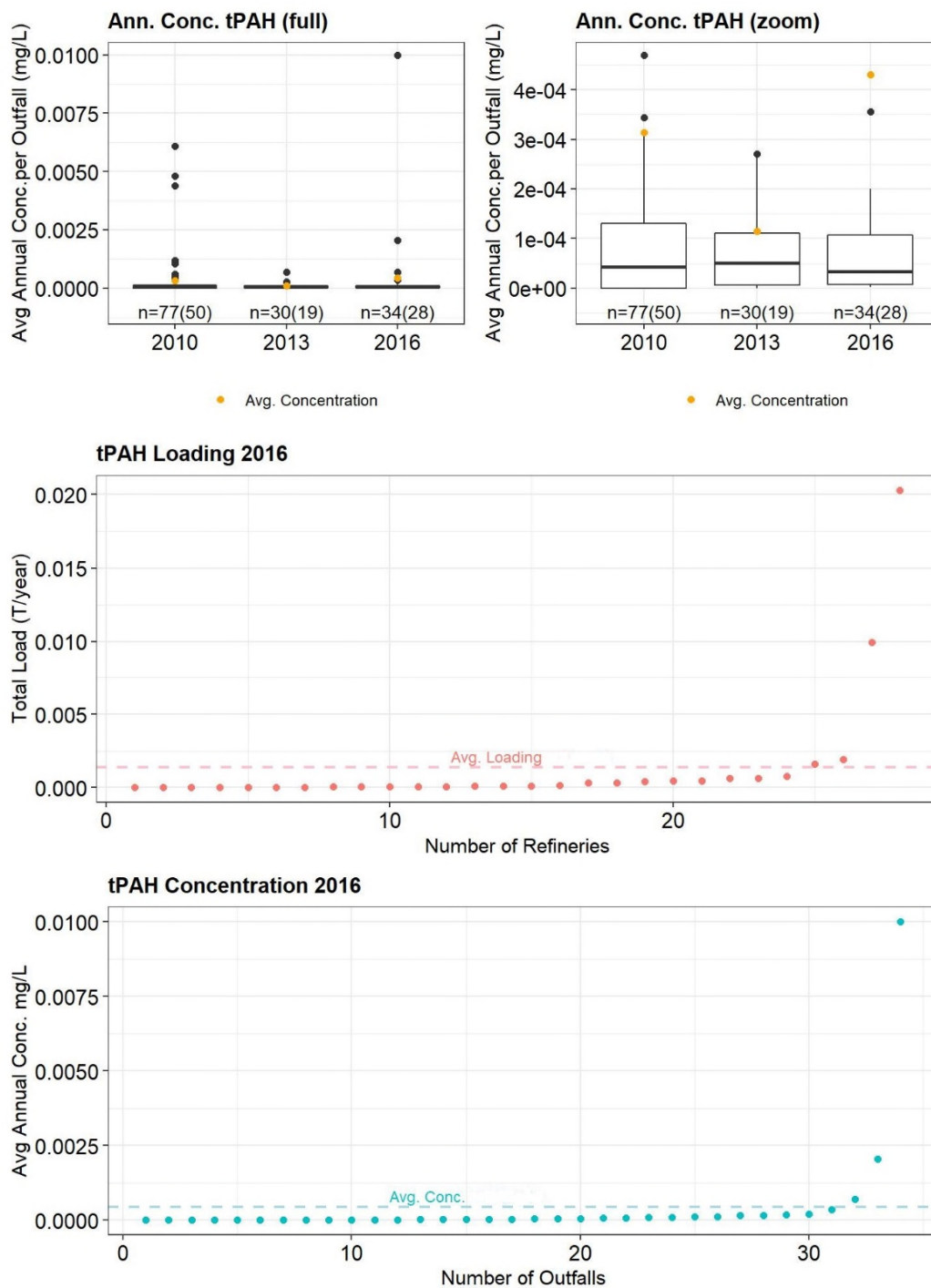
Figure 60. 2010, 2013 and 2016 survey results for total PAHs concentrations (two upper plots) and total PAHs total load and average annual concentration s-curves for 2016 (two bottom plots).
