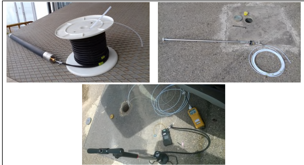
Figure 10. Vapor profiling methodology in piezometers.
