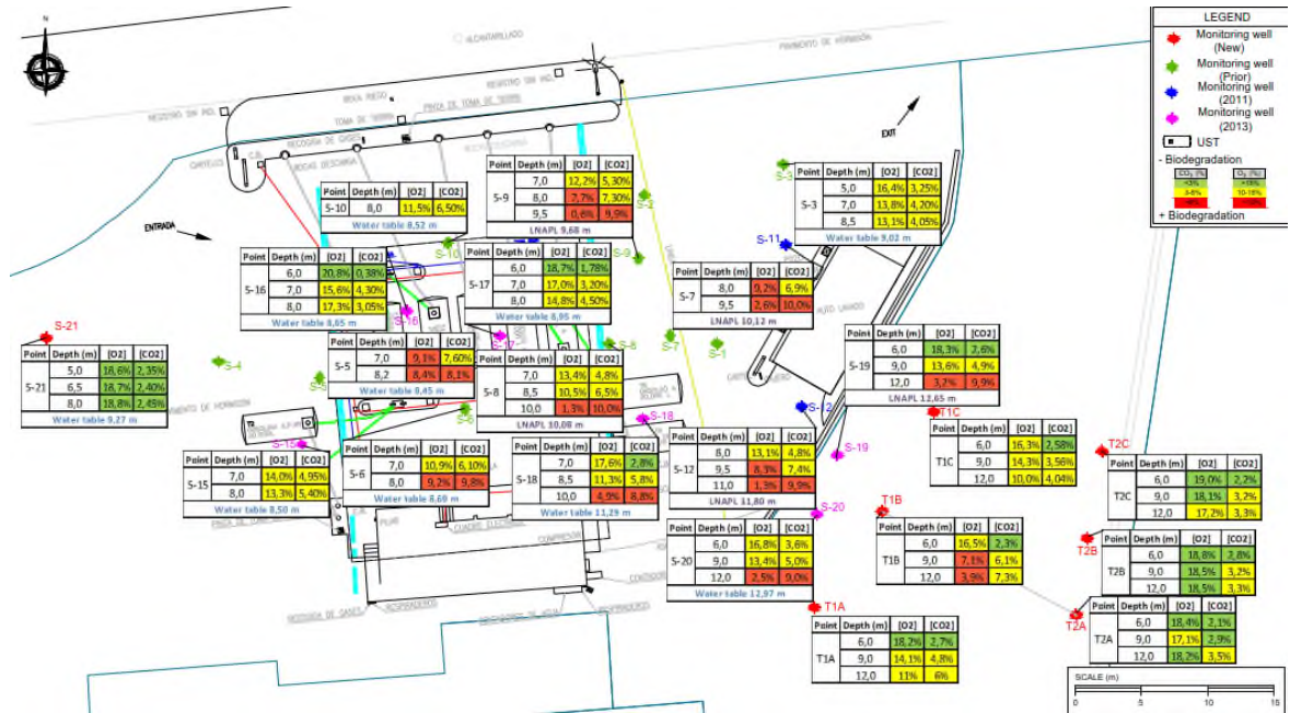
Figure 36. Results of O 2 and CO 2 Profiling in Monitoring Wells - January 2018
