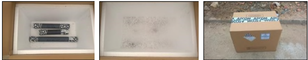
Figure 8. Preservation using dry ice and shipping of the undisturbed soil cores.
