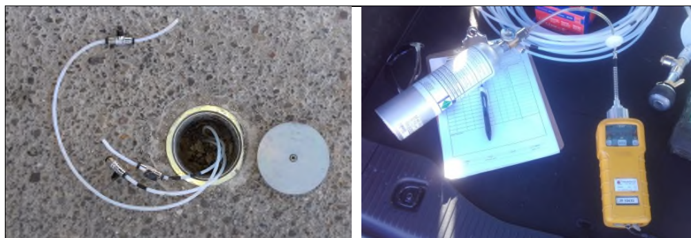
Figure 9. Vapor profiling methodology in SVPs
