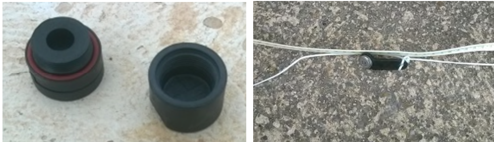
Figure 12. Temperature sensor installation.
