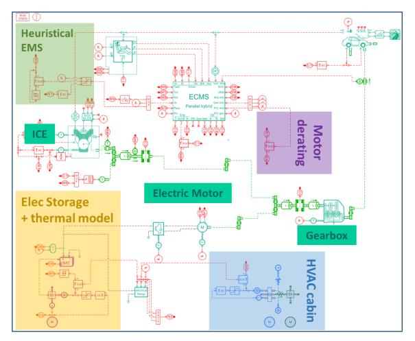
*Figure 52* Detailed Amesim sketch of P2 hybrid powertrain
