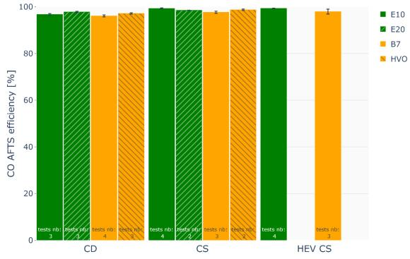
*Figure 32* Comparison of CO AFTS conversion efficiency [%] measured on RDE cycles on chassis dyno for each fuel and mode.
