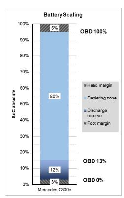
Such no-go zones and 80 % effective SoC range illustrated with next stacked bars seem consistent with protection margins and effective capacity benchmarked for latest Li-ion PHEVs.
