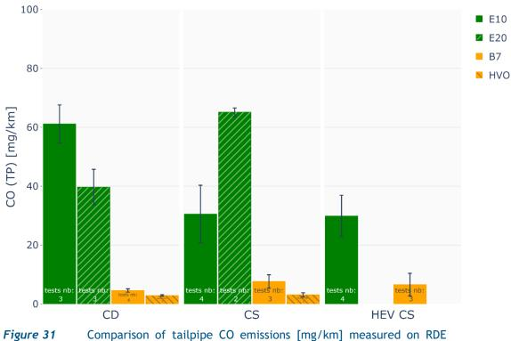
*igure 31* Comparison of tailpipe CO emissions [mg/km] measured on RDE cycles on chassis dyno for each fuel and mode.
