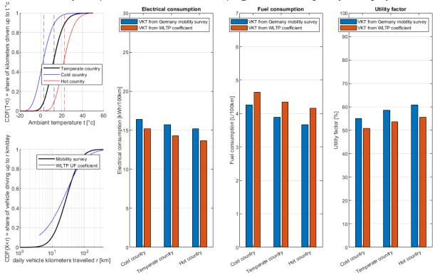
Sensibility to temperature and VKT distribition - example @15kWh and recharge every 2 driving days
