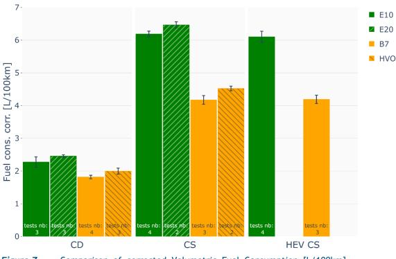
*Figure 7* Comparison of corrected Volumetric Fuel Consumption [L/100km] measured on RDE cycles on chassis dyno for each fuel and mode.
