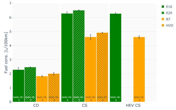
*Figure 6* Comparison of Volumetric Fuel Consumption [L/100km] measured on RDE cycles on chassis dyno for each fuel and mode.
