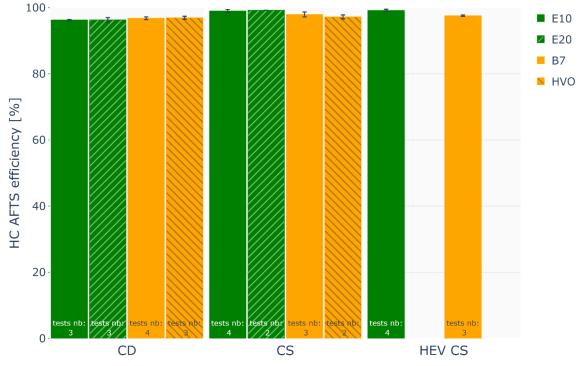
*Figure 35* Comparison of THC AFTS efficiency [%] measured on RDE cycles on chassis dyno for each fuel and mode.
