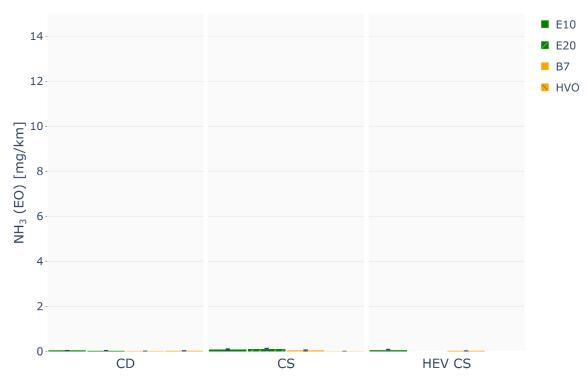
*Figure 36* Comparison of Engine-out NH<sub>3</sub> emissions [mg/km] measured on RDE cycles on chassis dyno for each fuel and mode.
