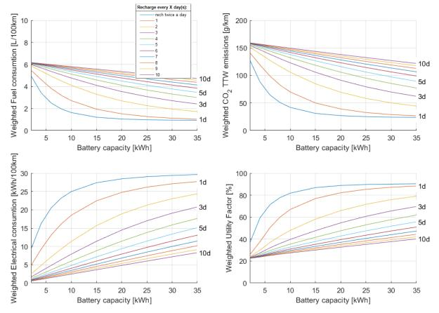
**Figure 88** Sensitivity of weighted average fuel consumption, CO<sub>2</sub> emissions, electrical consumption, and utility factor to the battery sizing and recharge period - Diesel vehicle
