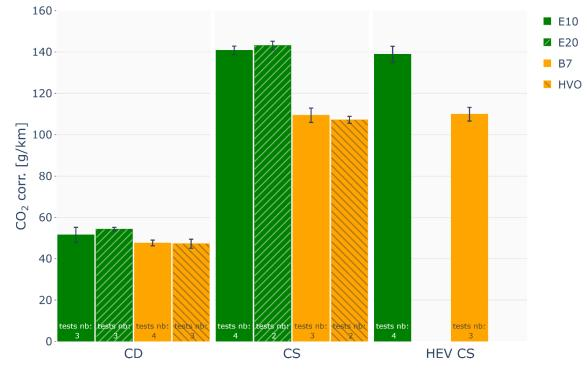
*Figure 12* Comparison of corrected tailpipe CO<sub>2</sub> emissions [g/km] measured on RDE cycles on chassis dyno for each fuel and mode.
