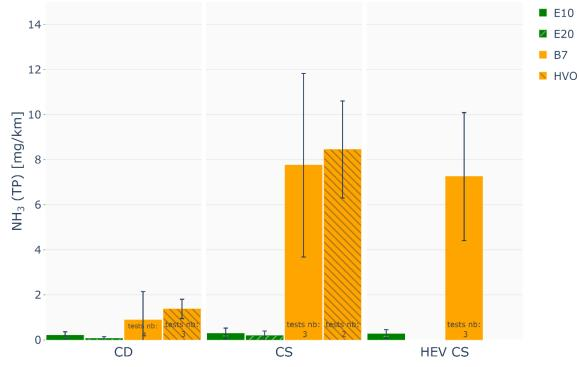
*Figure 37* Comparison of Tailpipe NH<sub>3</sub> emissions [mg/km] measured on RDE cycles on chassis dyno for each fuel and mode.
