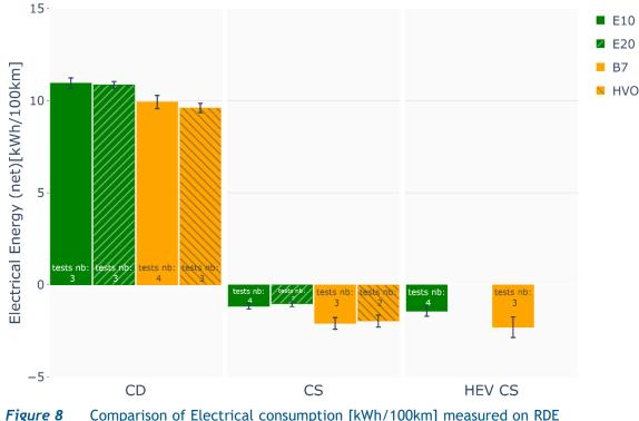
*igure 8* Comparison of Electrical consumption [kWh/100km] measured on RDE cycles on chassis dyno for each fuel and mode.
