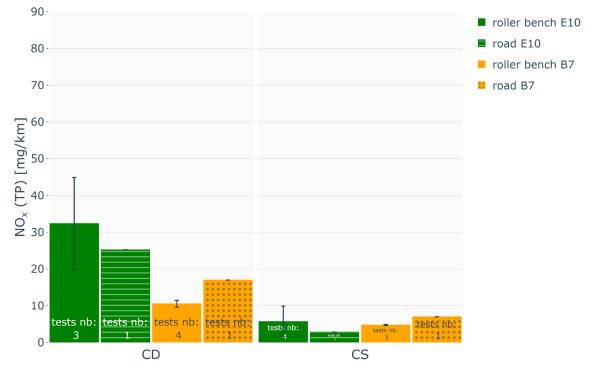
*Figure 48* Comparison of tailpipe NOx emissions [mg/km] measured on RDE onroad and chassis dyno tests for each fuel and mode.
