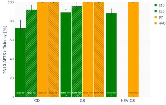
*Figure 26* Comparison of PN10 efficiency [%] measured on RDE cycles on chassis dyno for each fuel and mode.
