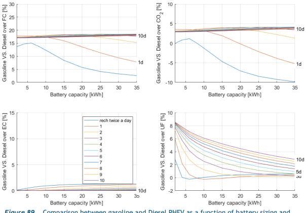
*Figure 89* Comparison between gasoline and Diesel PHEV as a function of battery sizing and recharge period
