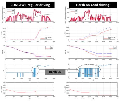
**Figure 60** Simulated CD comparison of standard CONCAWE cycle vs. harsh road driving - 1<sup>st</sup> row: speed cycle and cumulated distance - 2<sup>nd</sup> row: measured vs. simulated cumulated CO<sub>2</sub> emission (~fuel consumption) - 3<sup>rd</sup> row: measured vs. simulated battery SoC profile - 4<sup>th</sup> row: S equivalence factor profile for hybrid management - 5<sup>th</sup> row: modeled auxiliaries power demand profile
