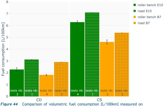
**gure 44** Comparison of volumetric fuel consumption [L/100km] measured of RDE on-road and chassis dyno tests for each fuel and mode.
