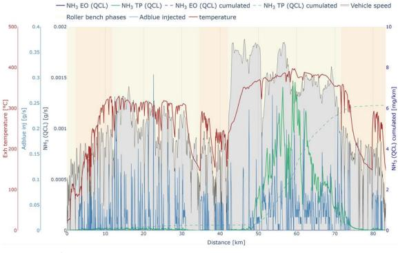
*Figure 38* Distance-based evolution of AdBlue injection, exhaust gas temperature and NH<sub>3</sub> emissions (EO and TP) along an RDE cycle.
