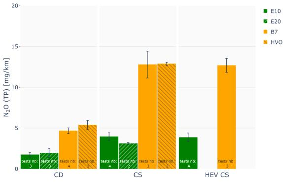
*Figure 17* Comparison of tailpipe N<sub>2</sub>O emissions [mg/km] measured on RDE cycles on chassis dyno for each fuel and mode.
