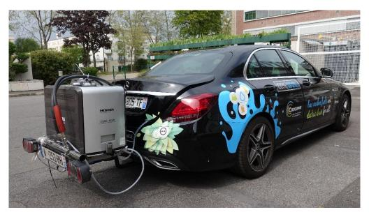
Figure 39 Vehicle setup for on-road tests, with PEMS equipment
