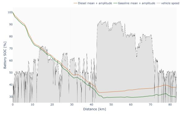
*Figure 46* Illustration of the battery SOC [%] evolution on road test in charge depleting mode
