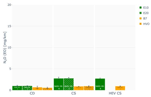
*Figure 16* Comparison of engine-out N<sub>2</sub>O emissions [mg/km] measured on RDE cycles on chassis dyno for each fuel and mode.
