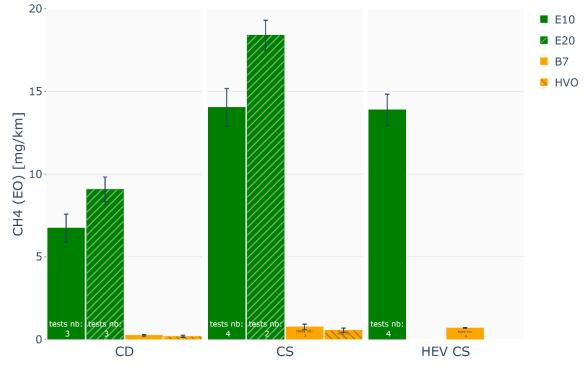
*Figure 14* Comparison of engine-out CH<sub>4</sub> emissions [mg/km] measured on RDE cycles on chassis dyno for each fuel and mode.
