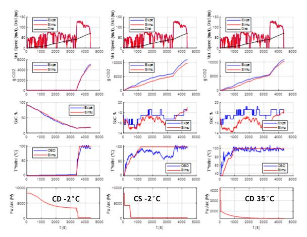
**Figure 57** CD and CS vehicle climatic tests simulation features - 1<sup>st</sup> row: speed cycle and cumulated distance - 2<sup>nd</sup> row: measured vs. simulated cumulated CO<sub>2</sub> emission (~fuel consumption) - 3<sup>rd</sup> row: measured vs. simulated battery SoC profile - 4<sup>th</sup> row: OBD vs. simulation engine water coolant temperatures - 5<sup>th</sup> row: modeled auxiliaries power demand profile
