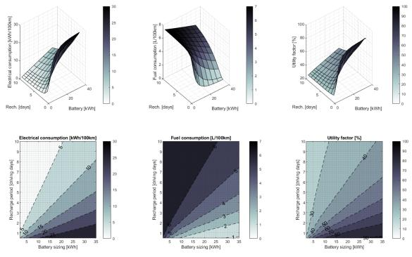
*Figure 82* Weighted average outputs on the full range of variation for recharge frequency and battery capacity
