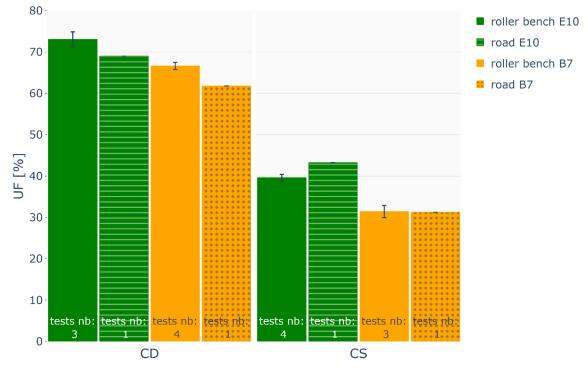
*Figure 47* Comparison of Utility Factor [%] measured on RDE on-road and chassis dyno tests for each fuel and mode.
