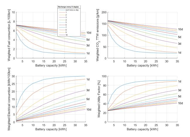
**Figure 87** Sensitivity of weighted average fuel consumption, CO<sub>2</sub> emissions, electrical consumption, and utility factor to the battery sizing (from 2 kWh to 35 kWh) and recharge frequency (from twice a day to every 10 days) - gasoline PHEV
