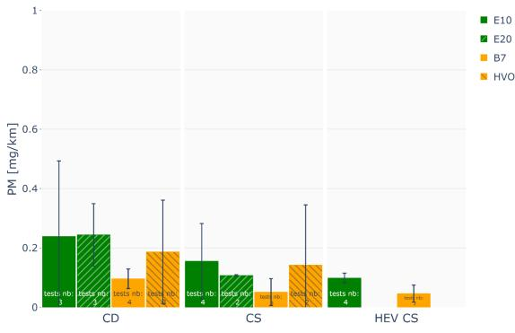
*Figure 29* Comparison of tailpipe PM emissions [mg/km] measured on RDE cycles on chassis dyno for each fuel and mode.
