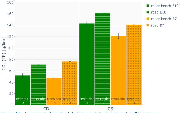
*Figure 43* Comparison of tailpipe CO<sub>2</sub> emissions [g/km] measured on RDE on-road and chassis dyno tests for each fuel and mode.
