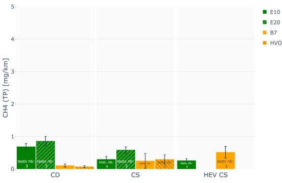
*Figure 15* Comparison of tailpipe CH<sub>4</sub> emissions [mg/km] measured on RDE cycles on chassis dyno for each fuel and mode.
