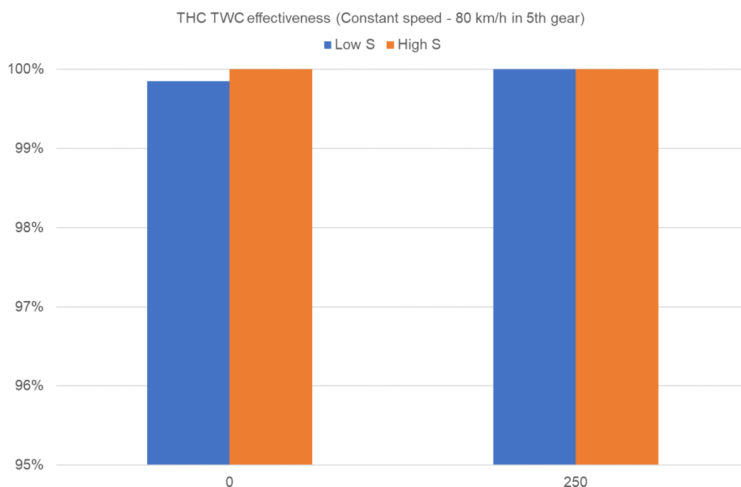
Figure 52 TWC conversion efficiency calculated from THC emissions results for TWC Low S, tested over the constant speed cycle.
