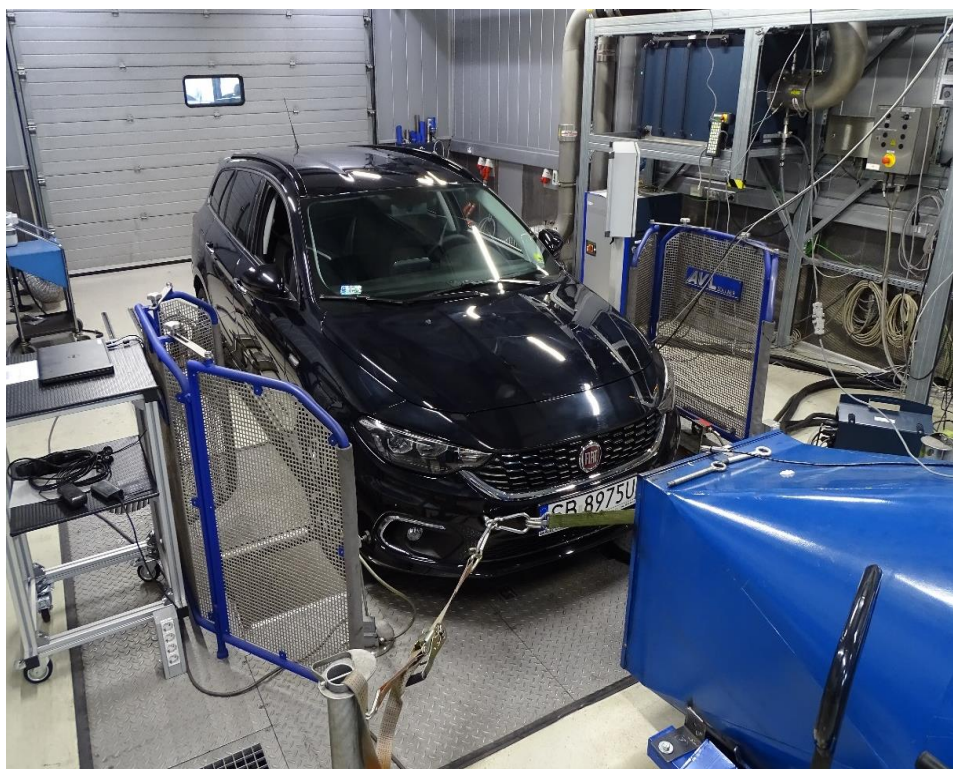
Figure 5 Fiat Tipo 1.4 bi-fuel vehicle during emission measurements in climate-controlled laboratory with an AVL Zöellner chassis dynamometer (2WD)
