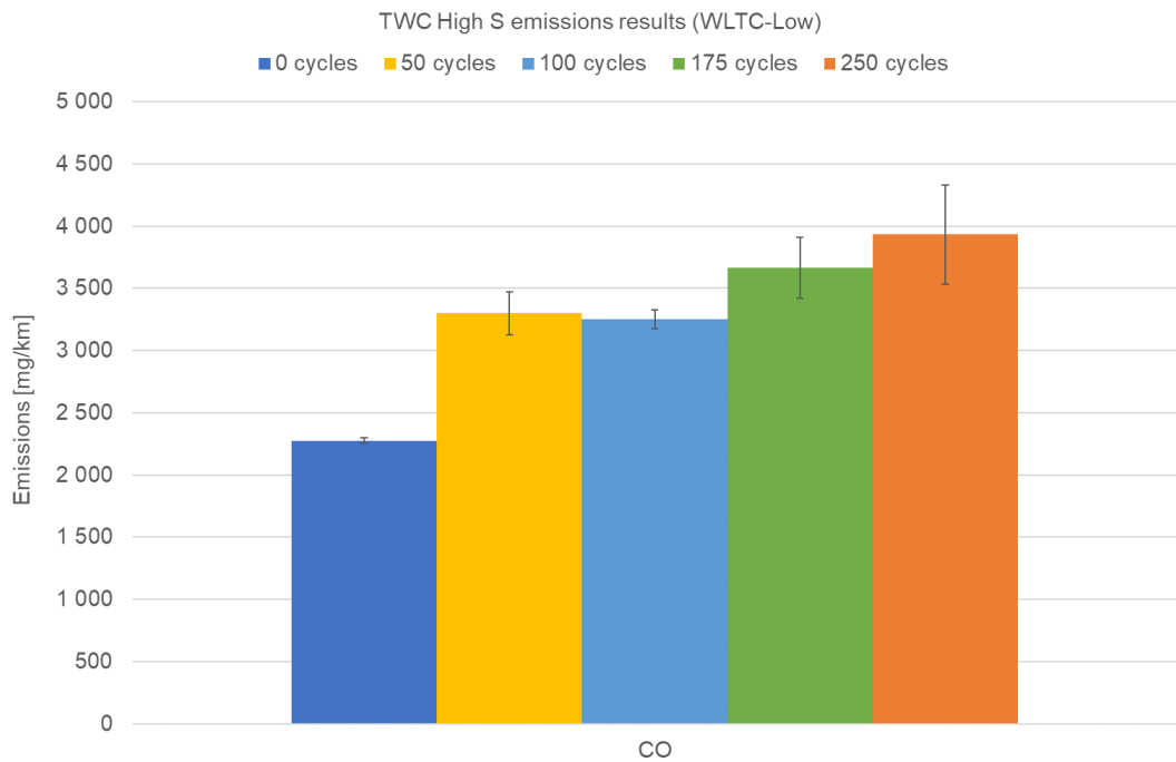
Figure 30 CO emissions results for TWC High S, tested over the Low phase of the WLTC.
