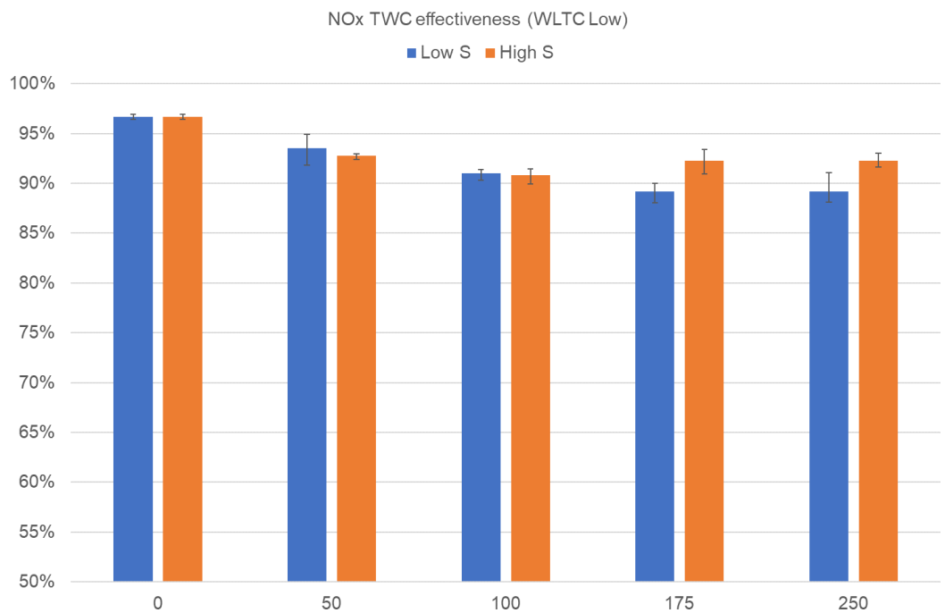
Figure 43 TWC conversion efficiency calculated from NO x emissions results for both test objects, tested over the Low phase of the WLTC.
