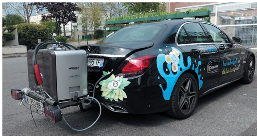
Figure 3: Vehicle set-up for on-road tests using a portable emissions measurement system
