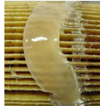
Biomass clogging a filter
