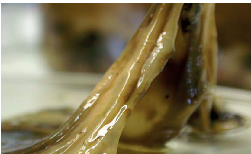
Figure 2 A typical biofilm that can be found in an affected fuel supply system
